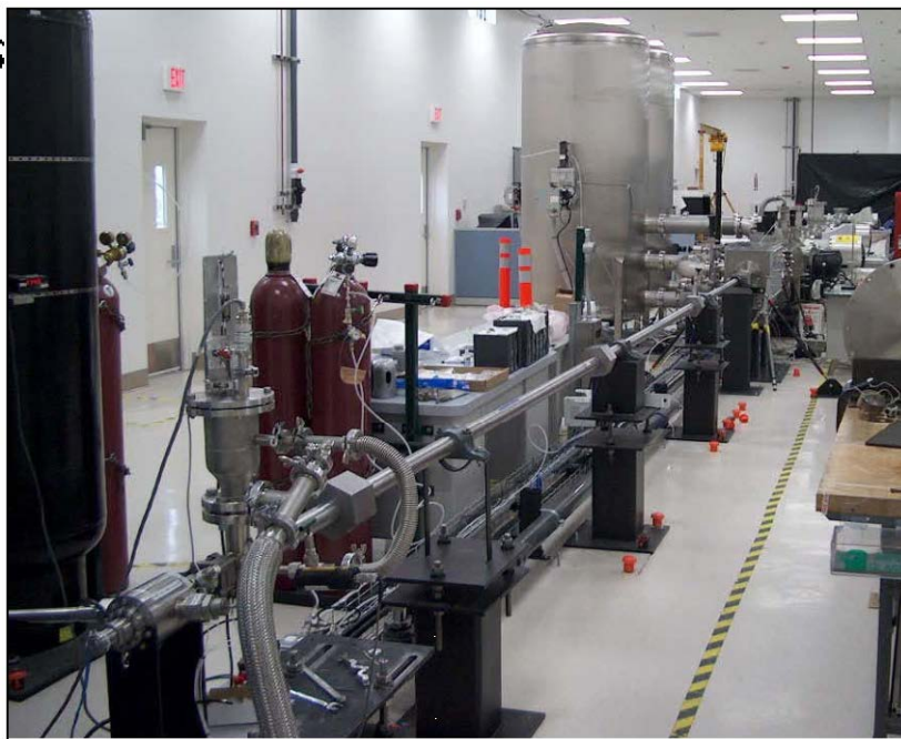
3335 3336 FIGURE 3.6 Inertial fusion energy target gas-gun injection experiment. SOURCE: 3337 General Atomics. 3338
